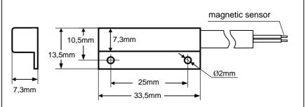
Fig. 1 Reed relay of K-1 magnetic contact in plastic housing
